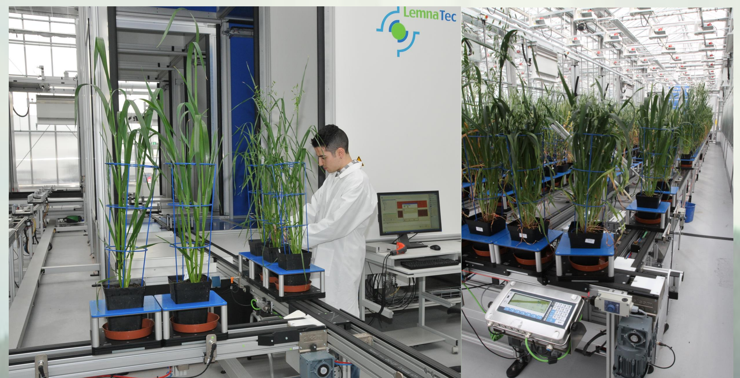
Automated greenhouse: imaging, watering, weighing
